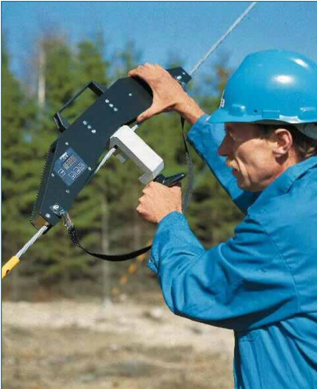
The PIAB RTM 20D can be used in applications where accurate measurement in pre loaded wire ropes is required. Such applications can be stay ropes, suspension ropes, catenary ropes etc. The PIAB RTM 20D is applied direct to the rope and the measured tension value is presented digitally.
