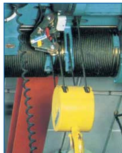
A typical installation of the PIAB LKV, installed at the anchor point of the hoist rope in a traveling crane. The PIAB LKV functions either as an over-load guard or as a slack line switch.
