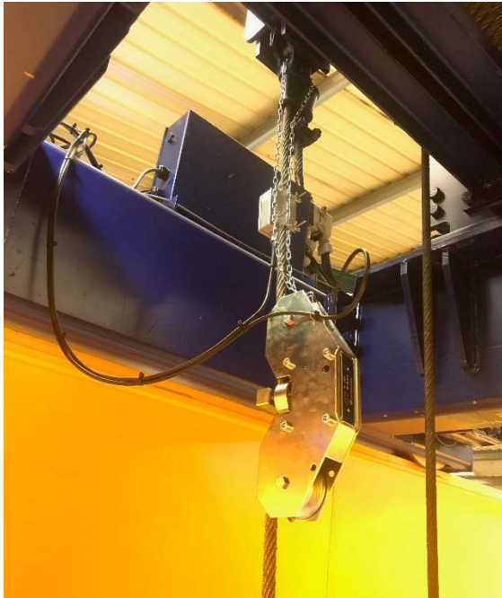
Picture: AMU sensor and LKVE force transmitter. Picture: 30-ton crane.
